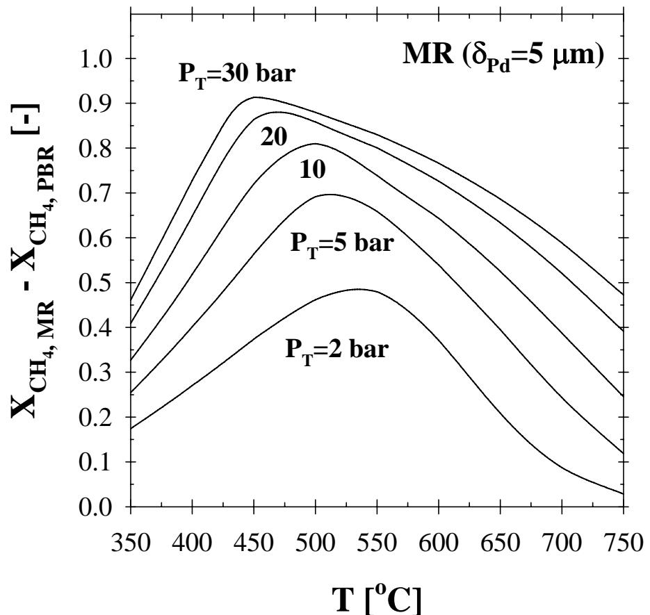
Maximum performance is achieved via the Membrane reactor (MR) at lower temperatures and high pressures.
