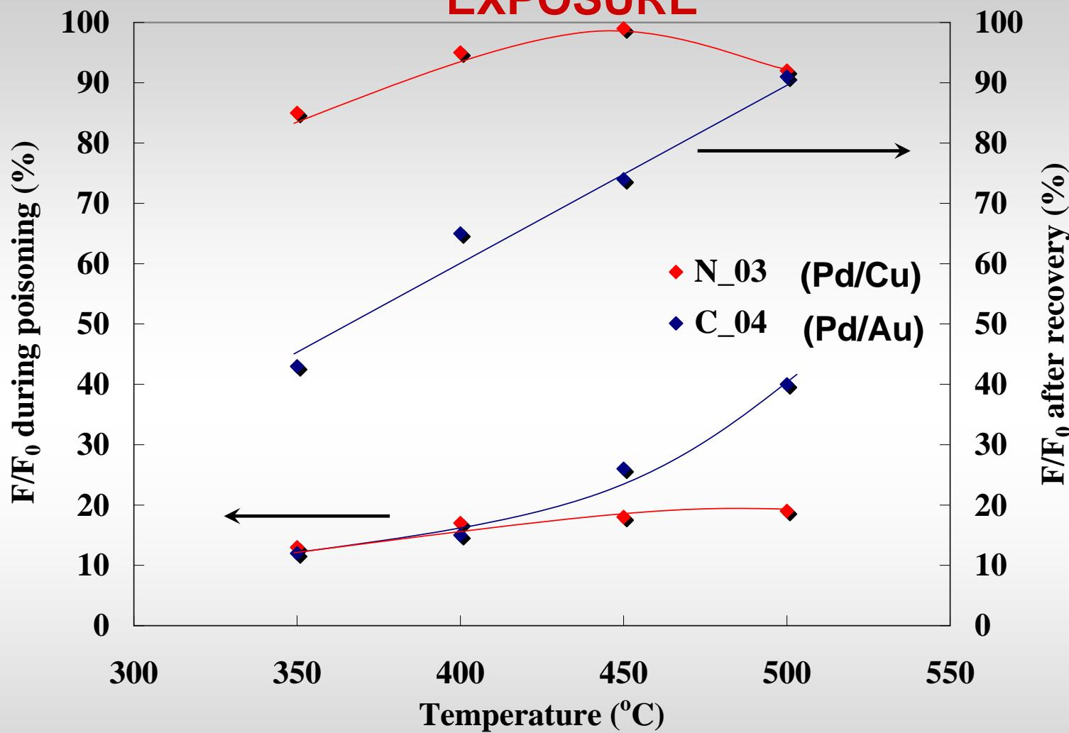
N\_03 and C\_04 were exposed to the H<sub>2</sub>S/H<sub>2</sub> mixture for 2 and 4 hour intervals, respectively, at each temperature. 14
