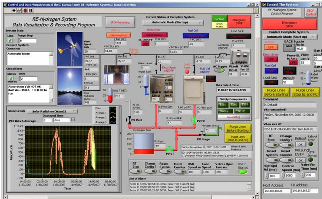
Figure 9. Data Visualization of the Kahua Ranch Installation (left) Available on a Web Site and Control Interface (right) only Accessible to Authorized Users.
