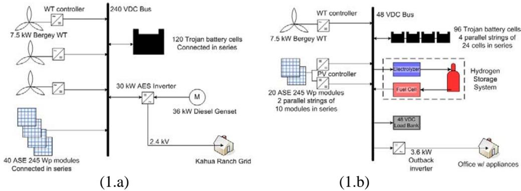
Figure 1. Design of the Installations at Kahua Ranch – (1.a): Village Power System; (1.b): Present RE-Hydrogen Power System.
