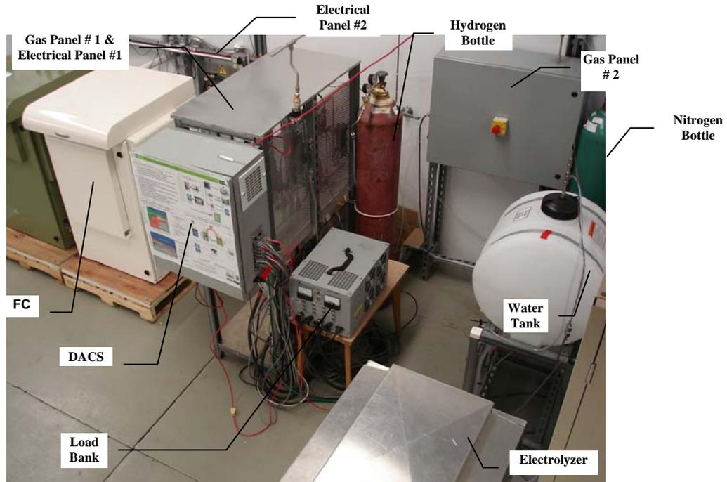
Figure 4. View of the Installation in Test at the HFCTF in Honolulu
