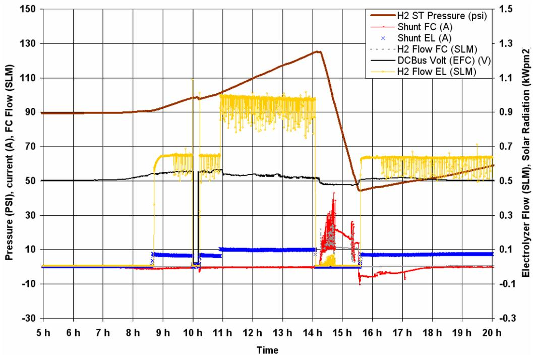
Figure 12. Evolution of the Hydrogen Storage System Data during a Day of Operation – October 5<sup>th</sup>, 2007
