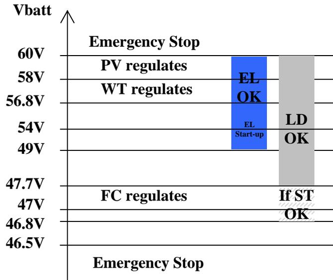
Figure 7. Voltage Control in the Overall Installation – Operating Voltage Range of the Components
