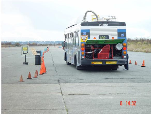
Figure 11. HCNG bus# 3302 undergoing emissions testing at the test track. The photograph also shows a simulated bus stop and blue marker barrels used to provide the driver with guidance on the point where a particular speed should be reached in order to adhere to the desired acceleration rate.
