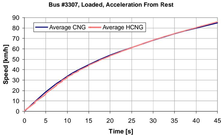
Figure 7. Bus#3307 CNG vs. HCNG acceleration comparison. Each curve represents the average of five runs.
