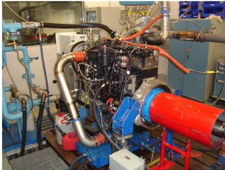
Figure 5. Engine as installed in the test cell for HCNG calibration.
