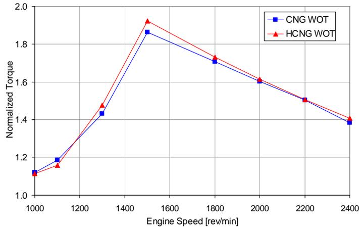
Figure 6. Engine torque curve comparison. The torque values are normalized against CNG torque at the lowest engine speed.
