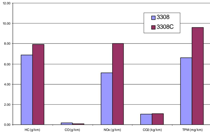
Figure 15. HCNG vs. CNG Bus Emissions in Transient Operation. 3308C designates the CNG operation of the bus
