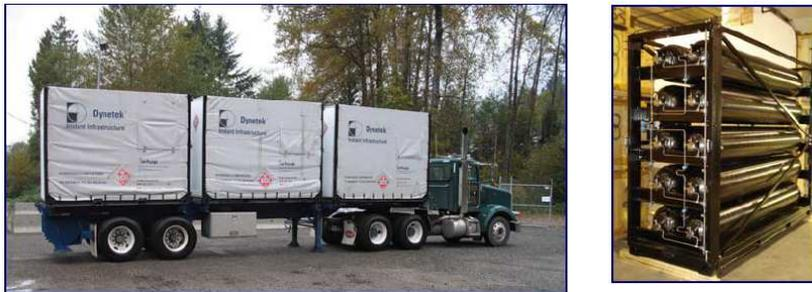
Figure 2. Hydrogen distribution trailer with PowerCubes.
