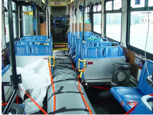
Figure 13. Inside of the HCNG test bus showing emissions measuring equipment at the back end and simulated passenger weight in terms of bags filled with water at the front end.
