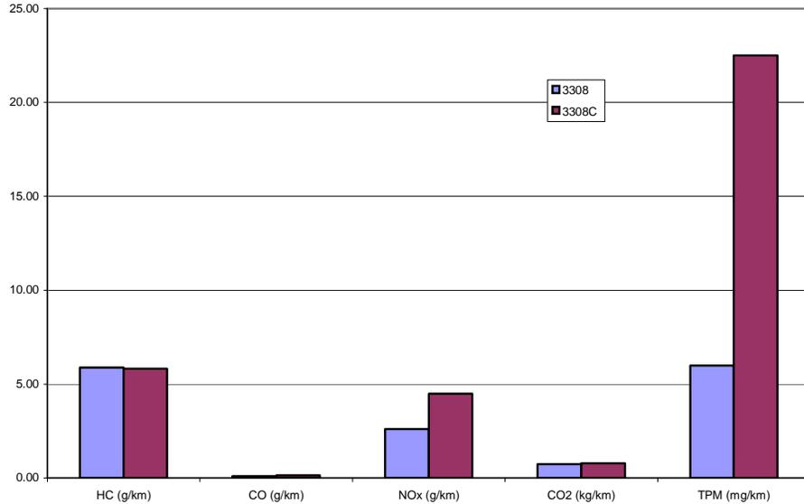
Figure 14. HCNG vs. CNG Bus Emissions in Steady State Operation. 3308C designates the CNG operation of the bus.
