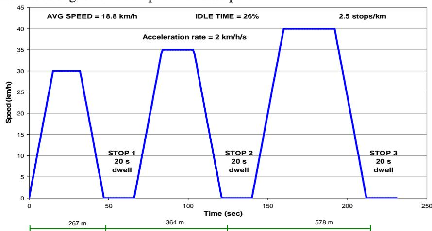
Figure 10. 2006 Emission Test Cycle.
