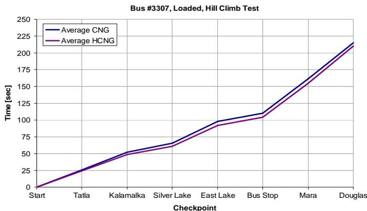
Figure 8. BU#3307 CNG vs. HCNG hill climb comparison. Each curve represents the average of four runs.
