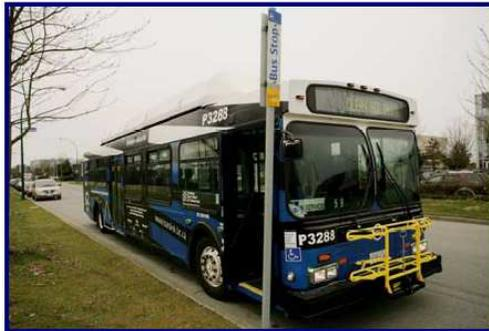
Figure 4. Heavy Duty HCNG Passenger Bus.
