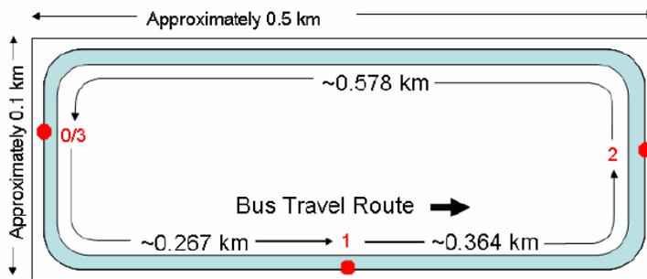
Figure 9. Bus emissions test track (2006).
