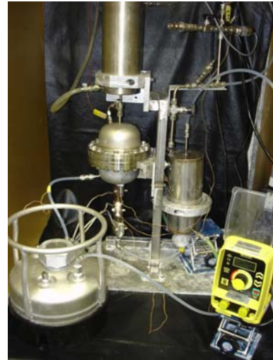
Figure 11. Batch BFR reactors: (a) 3L H 2 /hr, 0.5 hrs (b) 10L H 2 /hr, 8 hrs and (c) continuous flow reactor 100 L/hr
