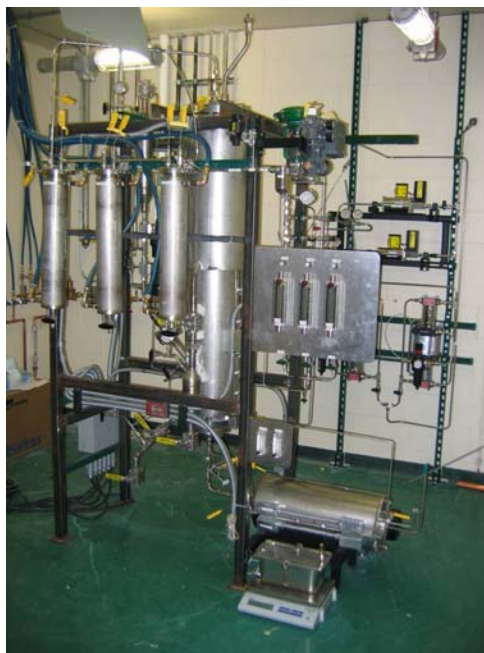
Figure 12. Prototype 10 kg H 2 /day solid biomass reactor
