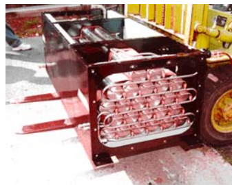
Figure 7 World's largest mobile metal hydride storage bed
