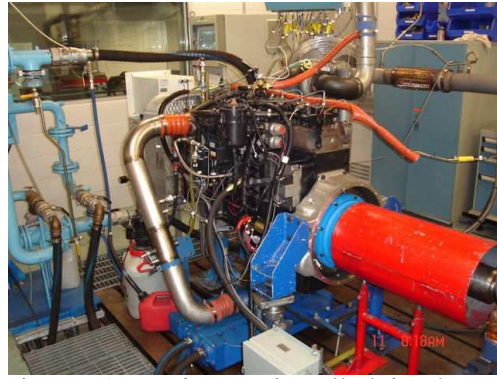
Figure 5. Engine as installed in the test cell for HCNG testing
