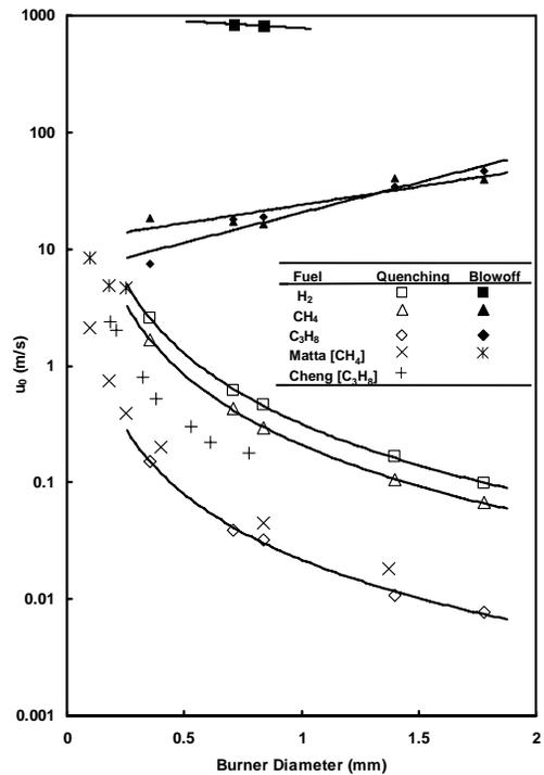
Figure 3. Measured fuel velocity at the quenching and blowoff limits versus burner diameter. The curves shown are fits of the present experiments.
