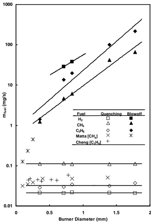
Figure 2. Measured fuel mass flowrate at the quenching and blowoff limits versus burner diameter. The lines are the fits of the present experiments.
