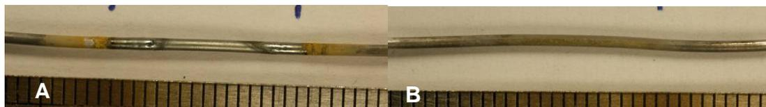
**Figure 5: Galvanized 1006-1008 Carbon steel following one hour of exposure to (A) hydrogen flame and (B) methane flame. The scale markings are in mm.**
