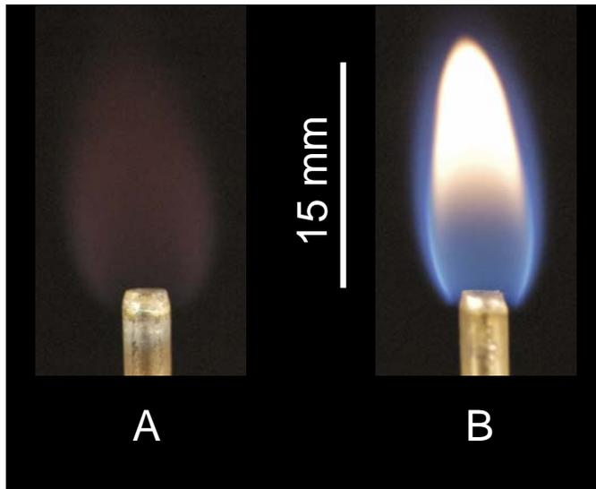
**Figure 1: Color images of (A) hydrogen flame and (B) methane flame.**
