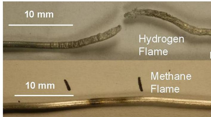
**Figure 4: Aluminum wires following 8 hours of exposure to (A) hydrogen flame and (B) methane flame.**
