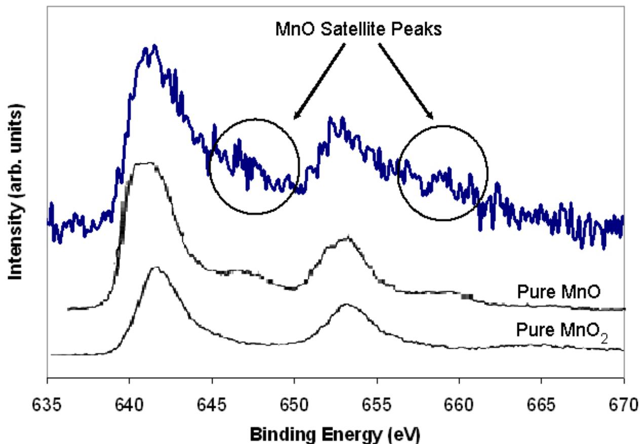
Mn 2p peaks show matching binding energies and satellite peaks corresponding to MnO (non-active).
