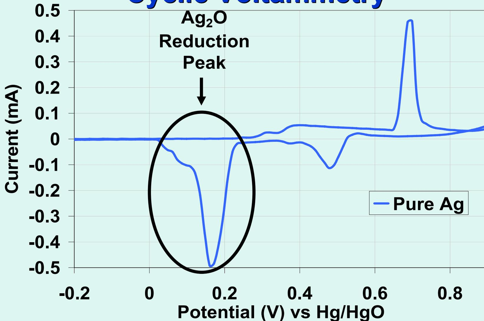
Sweep Rate: 500 mV / min, swept from -200 mV to 900 mV
